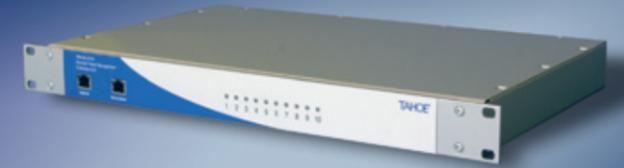
Tahoe 8116 is a cost-effective solution to extend the number of available power outlets of Tahoe 8216 Remote Power Management System. Each extension unit contains 10 additional sockets. Whole stack of Tahoe 8216 and Tahoe 8116 devices is controlled by the main Tahoe 8216 unit.
