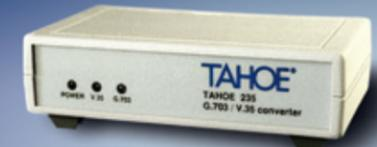
Tahoe 235 converter is equipped with one G.703 interface (2048 kbps, unframed) with RJ-45 connector and one V.35 interface with 34-pin Winchester connector.
